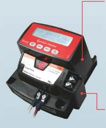
**The GeniSys Display** (Pt. No. 52067) allows a technician to monitor and program the primary control variables. The display shows current burner status, control timings, and burner cycle history. The display's programming mode allows a technician to customize both the pre-time and post-time settings and a lockout service message.
